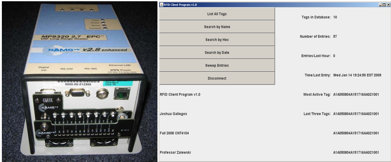
Fig. 3. RFID Device Employed in the Project (left) and the User Interface (right).
