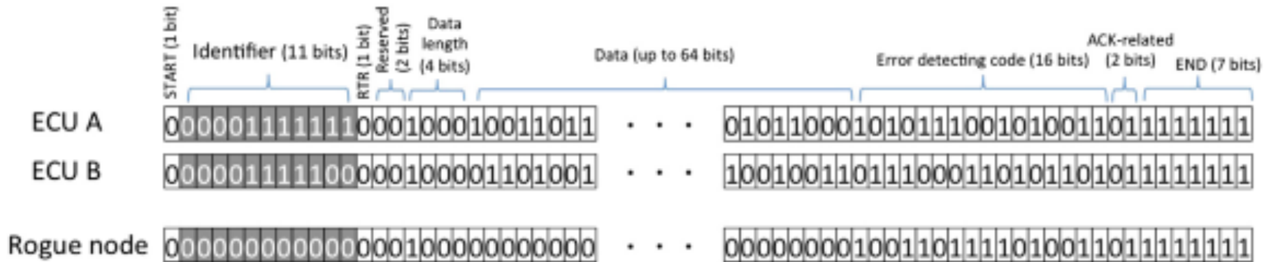
Figure 3.6 The structure of the standard CAN frame with up to 64 bits of data and 44 bits of overhead (identifier, error detecting code, etc.).
